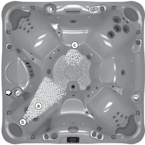
JET PUMP 1 – JET SYSTEM 1
